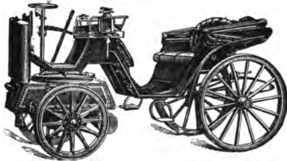
FIG. 58.—The Pretot Fore-Carriage shown attached to a Victoria Carriage. The attachment is on a fifth wheel running on roller bearings, and turning by geared connections with the steering hand wheel.
